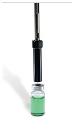
Figure 1: SPME fiber holder with fiber immersed into aqueous sample
