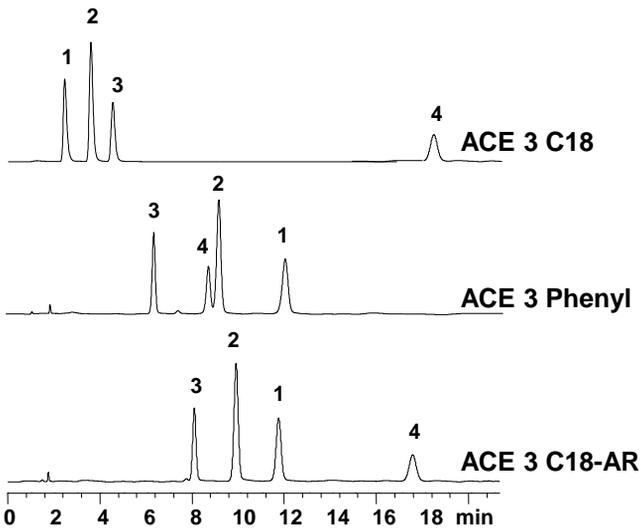
**Figure 4** Separation of substituted aromatic analytes, 1. TNB, 2. DNB, 3. NB, 4. Tol, 150 x 4.6 mm, MeOH/H<sub>2</sub>O 1:1 v/v, 1 mL/min, 40 °C, 210 nm
