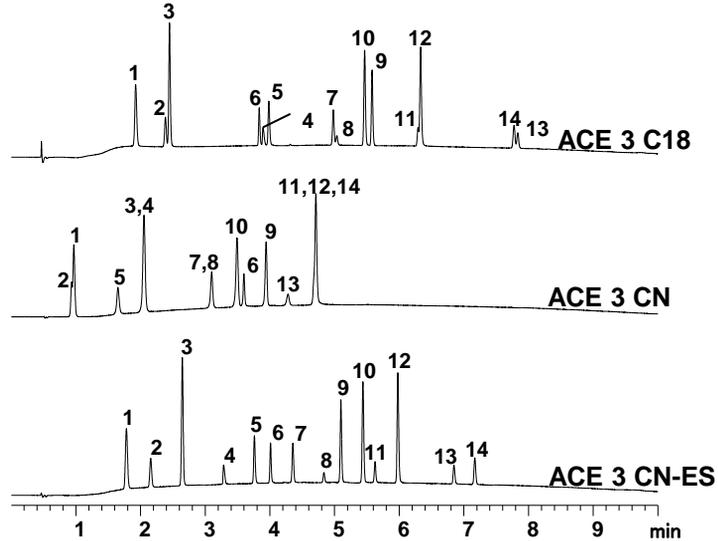
**Figure 5** Various compounds, 100 x 2.1 mm, A 0.1% formic acid in H<sub>2</sub>O, B 0.1% formic acid in MeCN, 3-100%B in 10 mins. 0.6 mL/min, 40 °C, 210 nm
