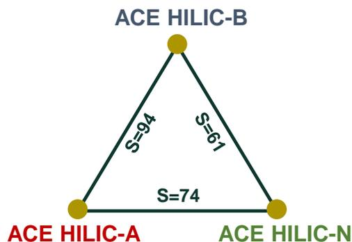
**Figure 2** Selectivity triangle for the ACE HILIC range using HILIC probes on 10 mM ammonium formate pH 4.7 MeCN/H<sub>2</sub>O (90:10 v/v)
