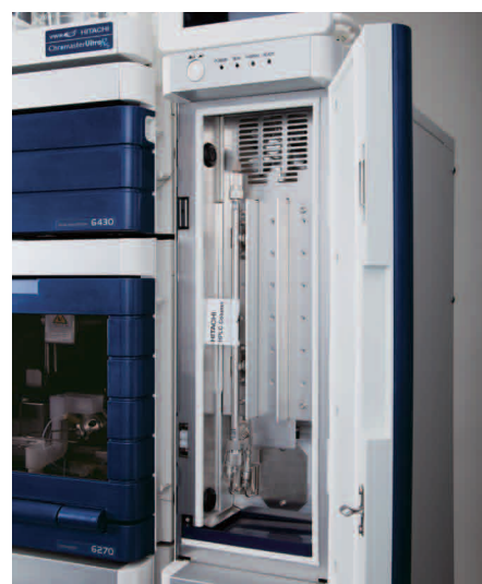
A view of column oven accommodating columns
