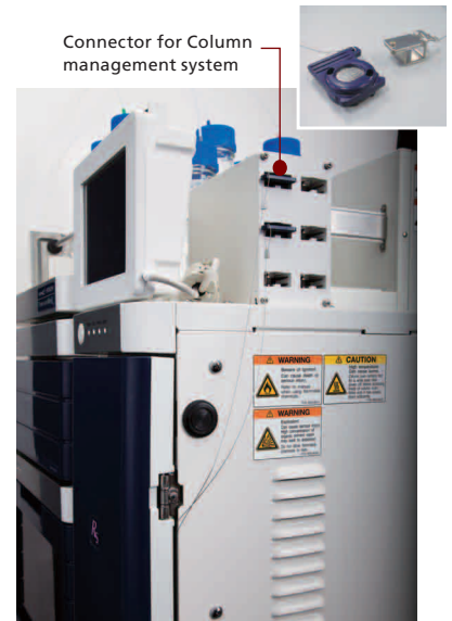
A view of connector for column management system connected
